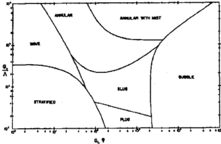
Figure 13: Baker's map for horizontal flow modified by Bell et al. (Bell et al., 1970).
