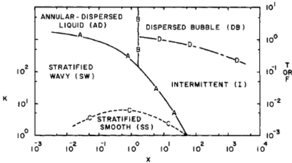
Figure 4. Taitel and Dukler's map for horizontal tubes (Taitel and Dukler, 1976).
