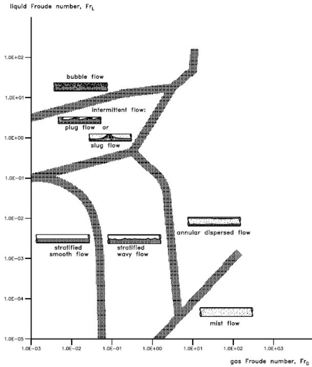
Figure 5. Shell's map for horizontal tubes (Shell company, 2007).
