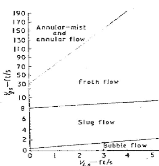
Figure 9: Golan and Stenning's map for up-flow (Golan and Stenning, 1969)
