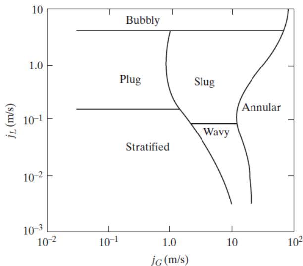
Figure 10: Mandhane-Gregory-Aziz's map for horizontal flow the upper one is the original (Mandhane et al., 1974), the second one is the same with SI units (Ghiaasiaan, 2008).
