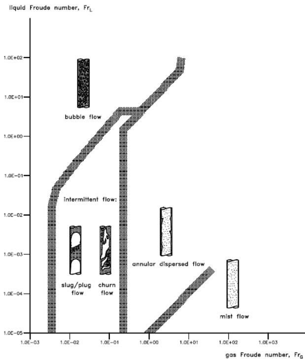
Figure 6. Shell's map for vertical tubes (Shell company, 2007).
