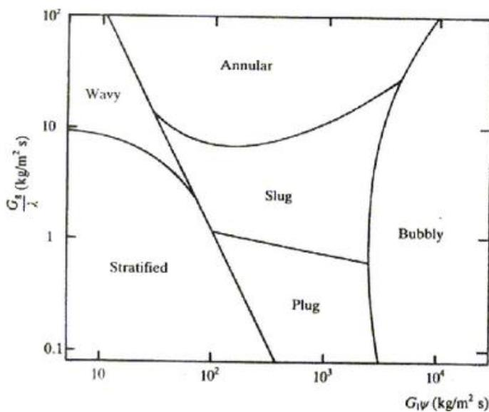
Figure 14: Modified Baker's map for horizontal flow (Whalley, 1987).
