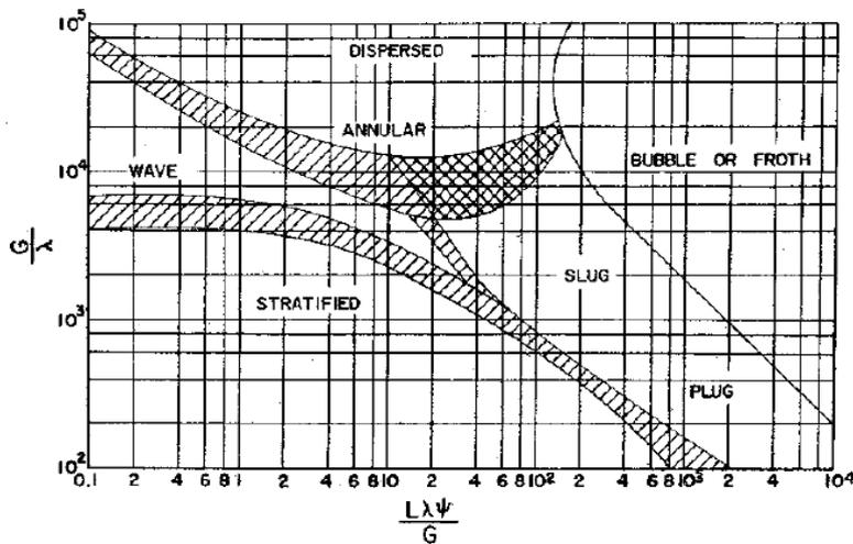
Figure 12: Modified Baker's map for horizontal flow (Scott, 1964).
