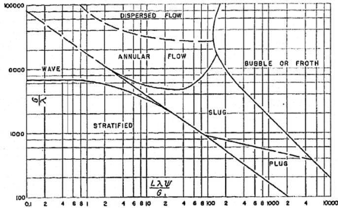
Figure 11: Original Baker's map for horizontal flow (Baker, 1954).
