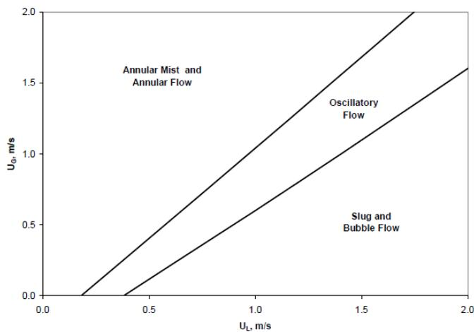
Figure 8: Golan and Stenning's map for down-flow in SI units (Pickering et al., 2001).
