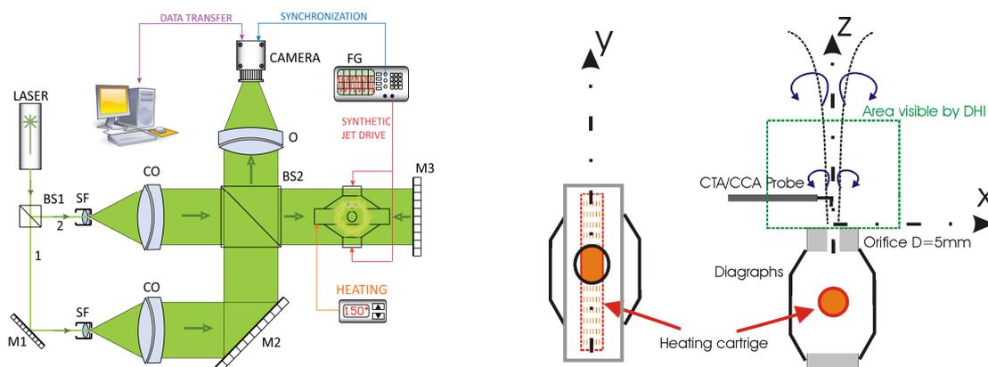
**Fig.1** (a) Setup for digital holographic interferometry with double sensitivity (BS-beam splitter, M-mirror, SF spatial filter, CO-collimating objective, O-focusing objective, FG-function generator), (b) A experimental device, system of coordinates and main dimensions for hot-wire anemometry and holographic interferometry
