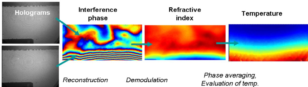
Fig.2 Steps for measurement of the temperature field by digital holographic interferometry
