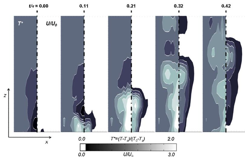
**Fig.3** Velocity (right side) and temperature (left side) fields at plane  $y=0$  at different times  $t/\tau$  of the cycle measured by CTA/CCA. The velocity field on  $+x, +z$  quadrant was measured due to the symmetry of the setup.
