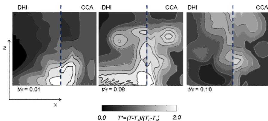
**Fig.4.** Temperature field above the jet. Images at different  $t/\tau$  achieved by digital holographic interferometry and CCA. The development of the jet is clearly visible from figures. Results from DHI represents average temperature field in  $y$  direction. Results from CCA are achieved at  $y = 0$ .
