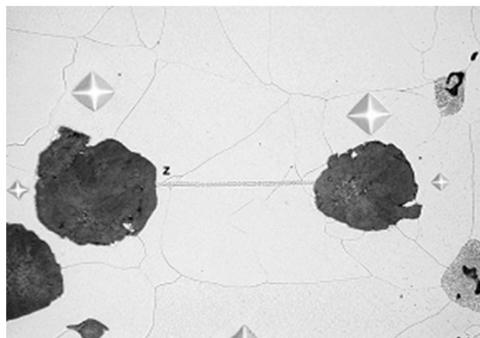
**Fig. 2** Structural characteristics measurement of ductile cast-iron ( $Z \equiv L_g = 165 \mu\text{m}$ )
