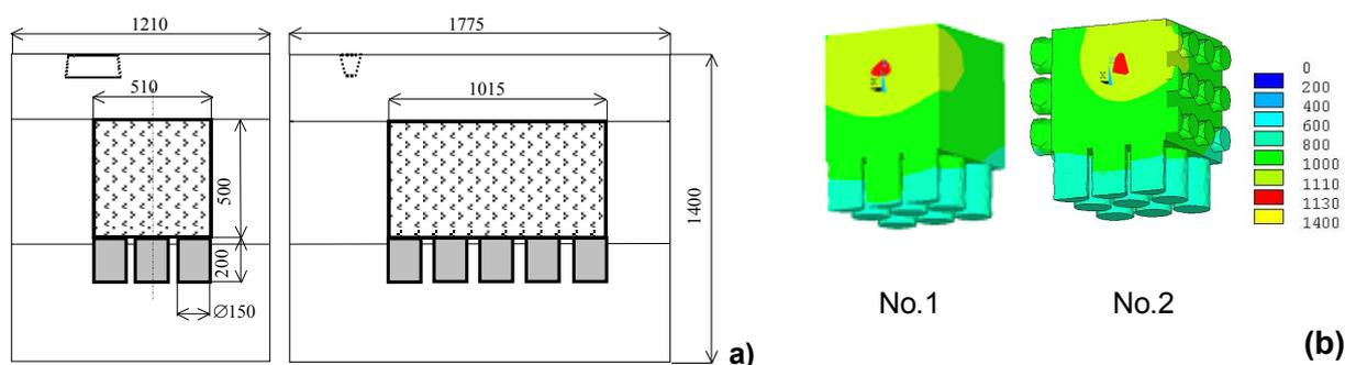
**Fig. 1 a)** The forming of casting No. 1 with chills on one side **b)** The calculated iso-zones in casting No. 1(5 hours) and No 2 (4.5 hours) and in its chills
