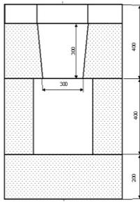
**Fig. 1** The casting-riser-mold system
