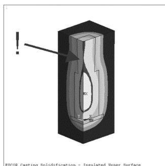
**Fig. 3** The temperature field of the system comprising the casting, the original riser and mold at 5200s
