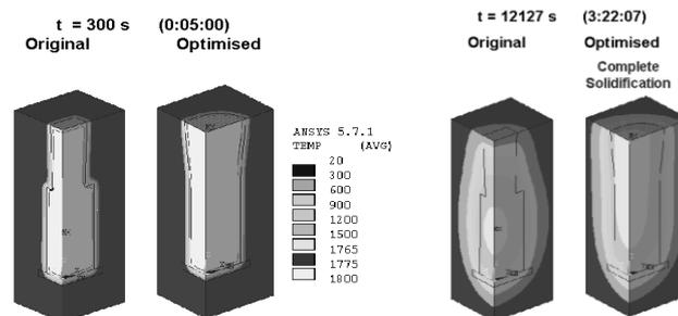
**Fig. 4** The temperature fields before and after optimization (300 s and 12127 s after pouring)
