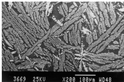
**Fig. 5** The structure of the sample B ( $L_B = 564 \mu\text{m}$ )
