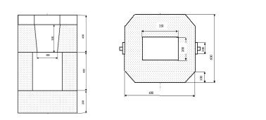
Fig. 1 The casting-riser-mold system
