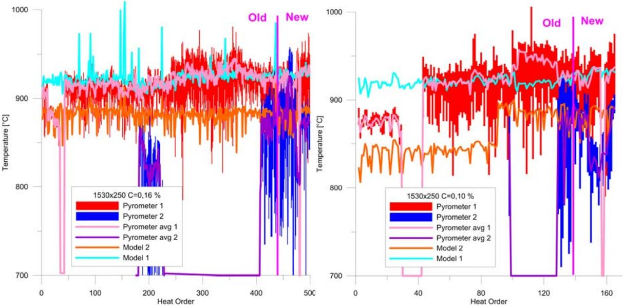
**Fig. 7** The measured and calculated temperatures of a 1530×250 mm slab
