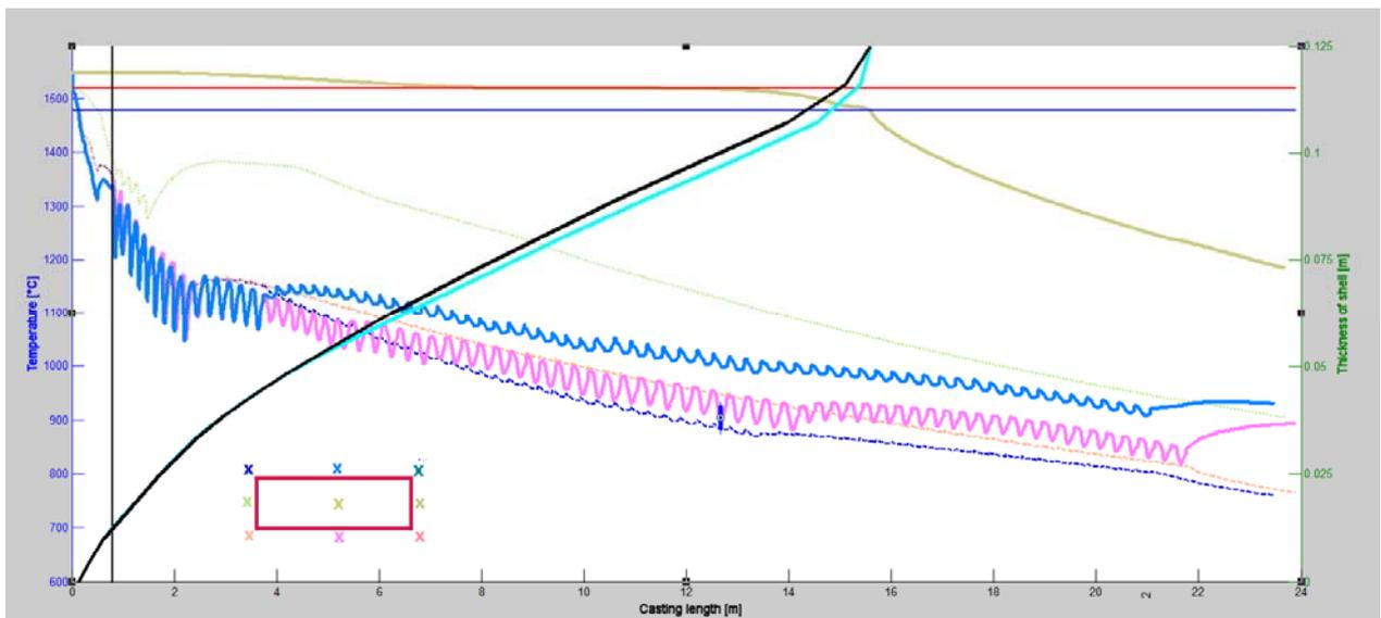
c) Nozzles 100.528.30.24 water flow per one nozzle 1.5 l/min
