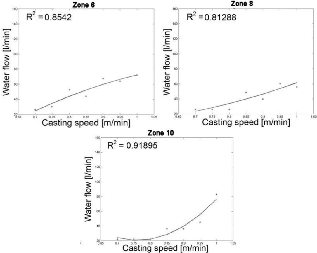
**Fig. 8** The optimal cooling curve for cooling zone with new nozzle
