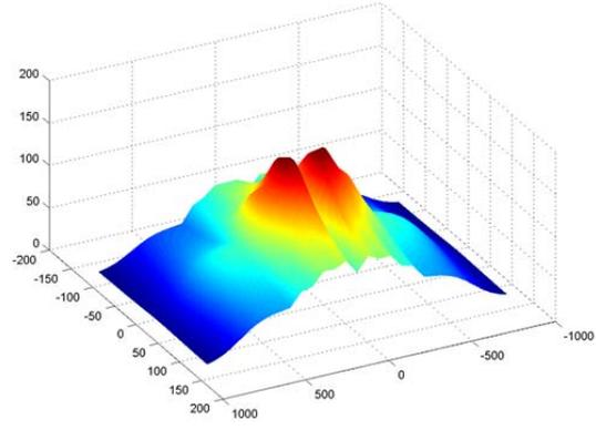
b) Nozzle 100.528.30.24 water flow 2.2 l/min, air pressure 0.2 MPa
