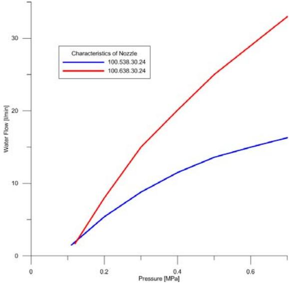
**Fig. 2** Characteristics of nozzles Lechler 100.638.30.24 and 100.528.30.24
