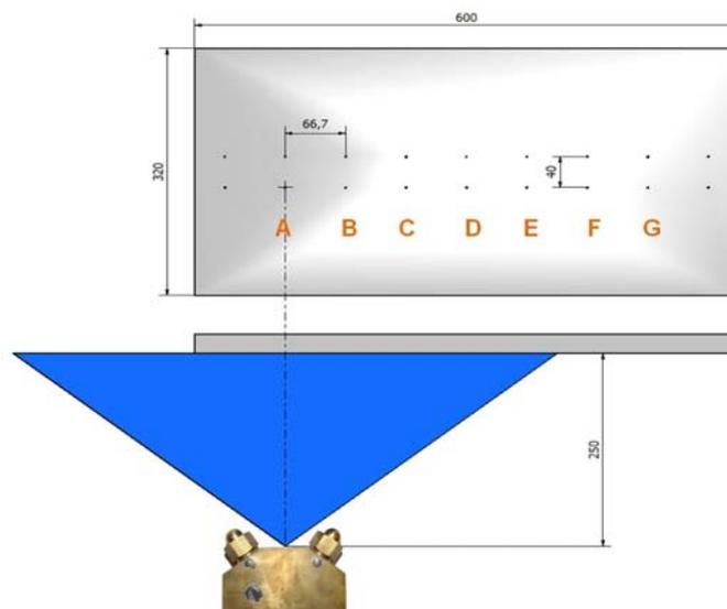
**Fig. 3** Diagram of measurement configuration of the cooling effects of nozzle
