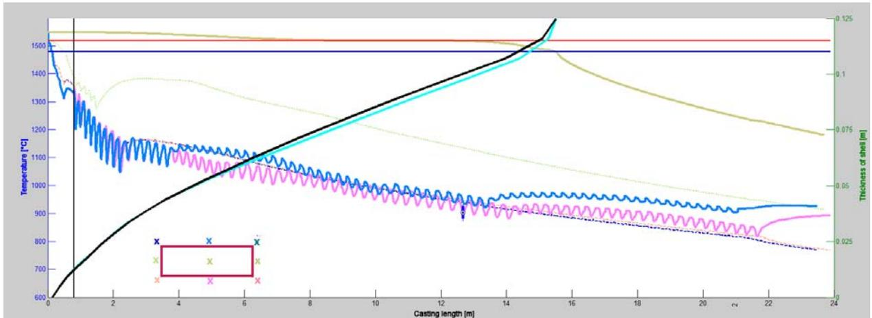
a) Nozzles 100.638.30.24 water flow per one nozzle 2.2 l/min
