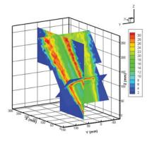
■ Turbulence intensity in a jet issuing from an air terminal device
