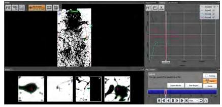
Particle tracking software Photron FASTCAM Analysis used for droplets tracking in the spray generated by a twin-fluid atomizer. Operating pressure 70 kPa, gas-to-liquid ratio 5%, recording frequency 42,000 fps, shutter 22.8 µs, resolution 480 × 1024 pixels.
