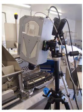
A high-speed videorecord of artificial casing filling.
