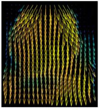
Evaluation of the velocity field of the spray generated by the pressure swirl atomizer using Particle Image Velocimetry algorithms. Operating pressure 235 kPa, camera recording frequency 96,000 fps, shutter 0.25 μs, resolution 768 x 512 pixels.
